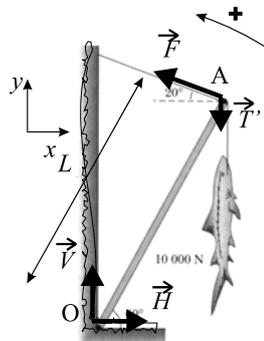
$$\begin{aligned} -F \cos 20^\circ + H &= 0 \\ F \sin 20^\circ - T' + V &= 0 \\ F \sin 20^\circ - T' \sin 20^\circ &= 0 \end{aligned}$$
